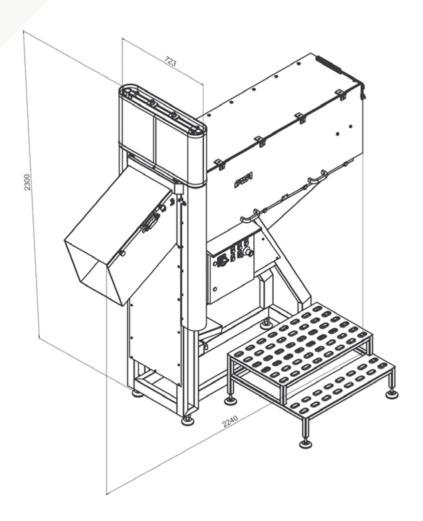
**SLP** is designed to cut 10-25 kg butter blocks into small pieces before homogenizing and re-packaging of butter.
