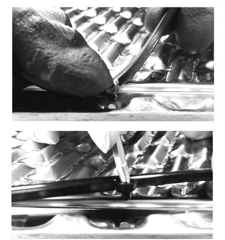
• on the backside of the plate, the burlings have to be visible
