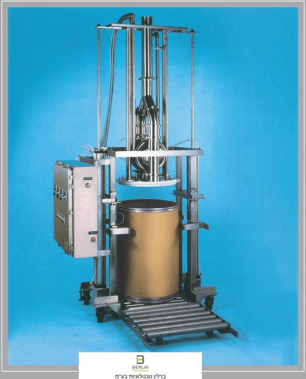
ברלין טכנולוגיות בע"מ שדרות גן רווה 13, יבנה, 8122214 http://www.berlintech.co.il/ mail@berlintech.co.il טלפון: 073-7597171 פקס: 08-6638120 The Murzan DUS-50 is the ultimate solution for emptying the most viscous materials from 55-gallon drums or containers of any shape. When used in applications which no pump alone could handle, the system empties the containers quickly and cleanly without adding any pressure to the product or the container. The system is FDA listed and USDA approved.
