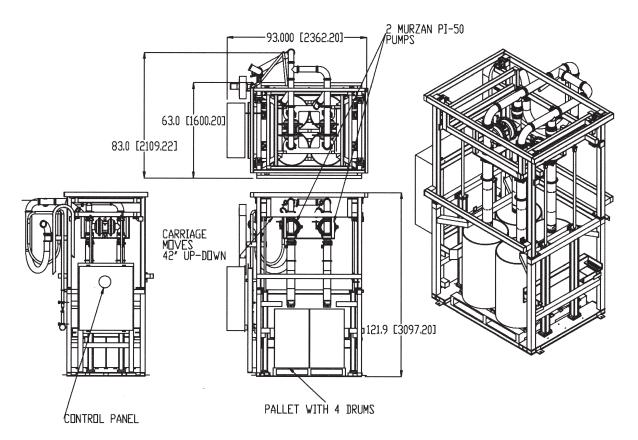
The Murzan ABDT juice concentrate unloading system consists of two double diaphragm pumps that are mounted on a stainless steel carriage that moves the pumps and suction wand up and down to allow entrance and unloading of the four drums on a pallet at the same time.
