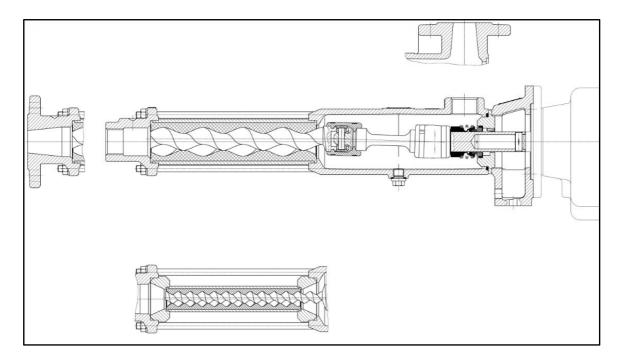
This flexibility enables a flow rate variation by simply exchanging conveying elements without requiring cost intensive refurbishments and installation adjustments such as piping modifications etc.
