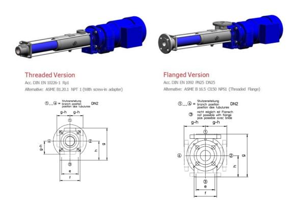
To achieve broad market coverage, the pump casings will be made of high-grade stainless steel. This material choice allows the pumps to be used in a broad range of applications. By default, the suction casing has three additional closed drillings in order to ensure a flexible use of the pump. The suction casing can be turned by 90°, while still allowing the pump to be drained safely. In addition, these connections can be used to add sensors, flush or fill the pump.
