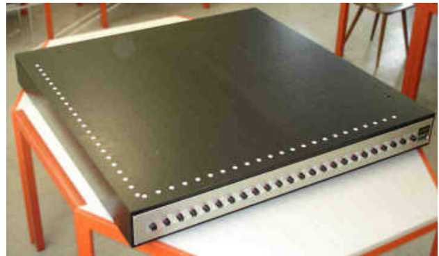
Temperature measuring board, 23 x 23 = 529 measuring points
