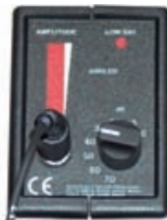
Visual leak warning
