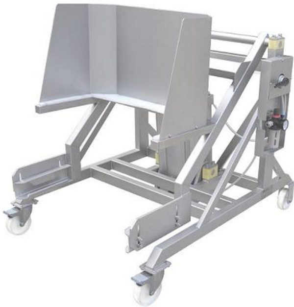
Swing loader for lifting and turning of 200L trolleys - carrying capacity up to 350 kg - pneumatic drive 30.2104.00
