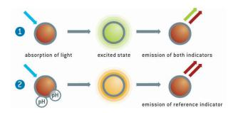
pH Microsensors are miniaturized pH sensors designed for measuring in small volumes and high spatial resolution. The sensor tip is below  $150\,\mu\text{m}$ . The sensors are based on a  $140\,\mu\text{m}$  silica fiber which enables integration into a manifold of small scale environments. These sensors do not require reference electrodes and there is no leakage of electrolytes, a clear advantage over common electrodes.
