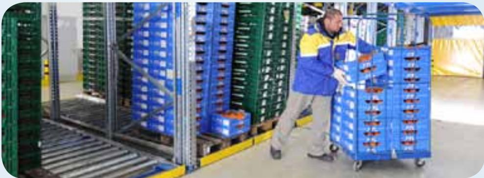
Gravity roller conveyors and live storage system for pallets lengthways and crossways transport
