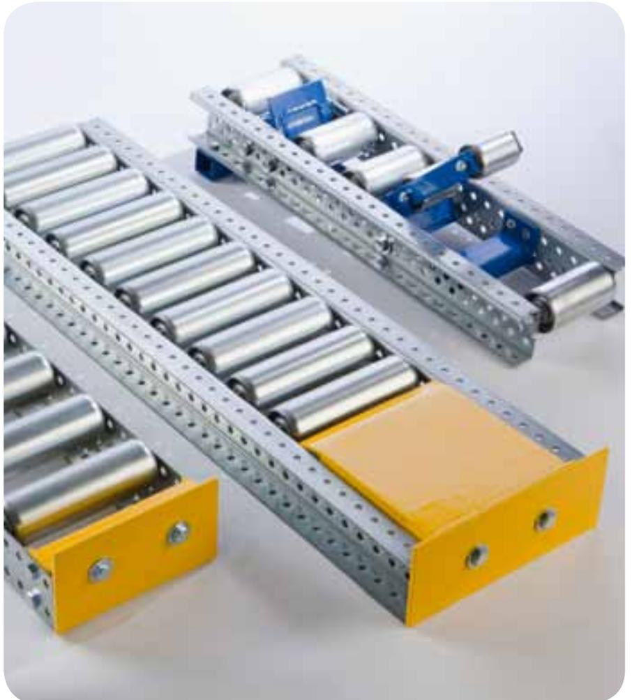
Standard lengths are 2496 mm and 6500 mm. Other required lengths can, of course, be supplied. Longer tracks are connected with connecting rods. Please choose the track length in a pitch of 26 mm. Tracks can be equipped with wheels in a pitch (T)
