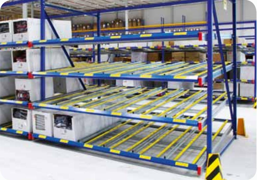
Fix and Autofix-Wheel Rails used in picking location
