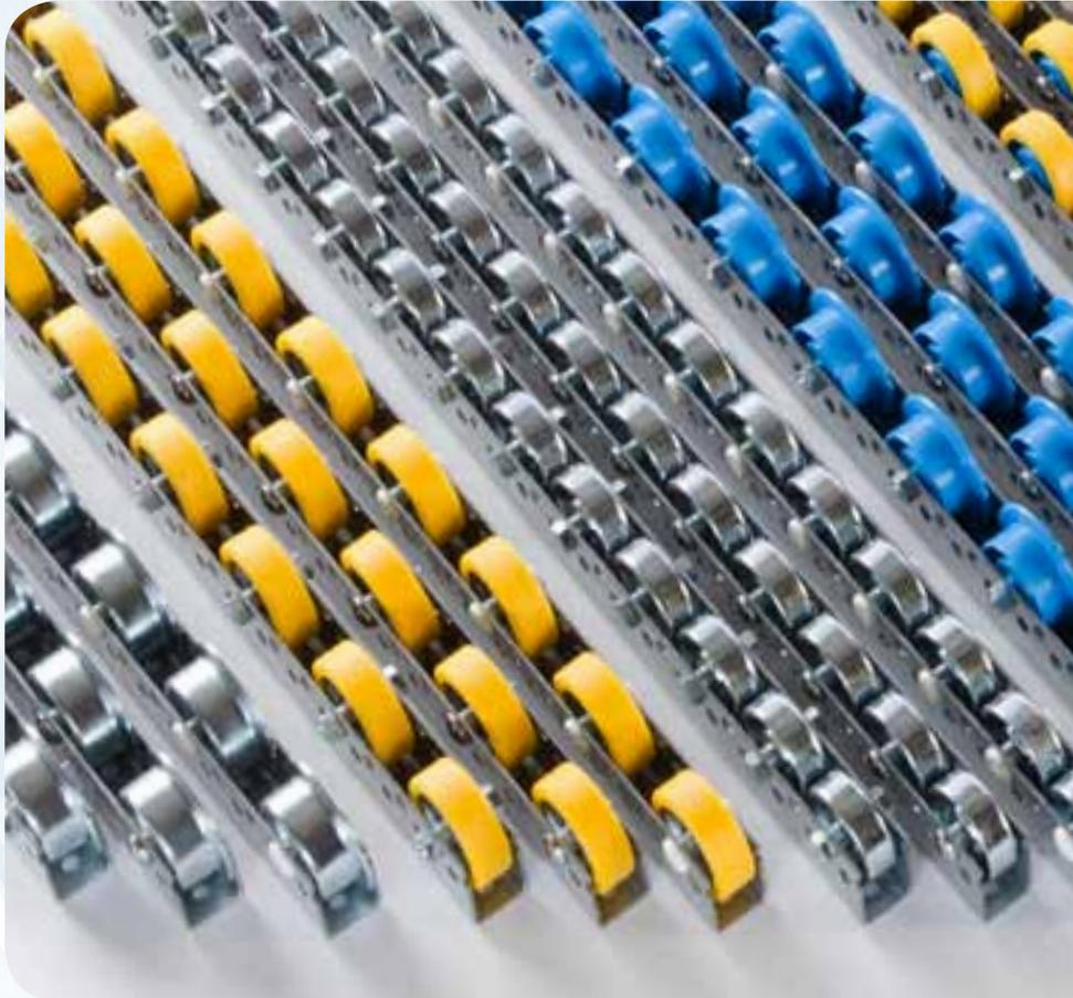
The Universal Roller Tracks consist of a Sendzimir-galvanised steel profile at a gauge of 2 mm thickness. The profile has 2 sets of lateral perforations at different heights at a pitch of 25 mm, the base is also punched with holes at a 25 mm pitch. The diameter of the holes is 8.1 mm.
