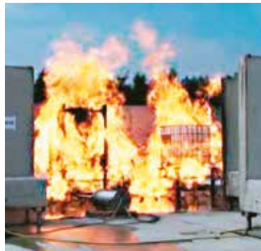
Stainless steel vs. Plastic: Fire resistance test at the Federal Institute for Materials Research and Testing
