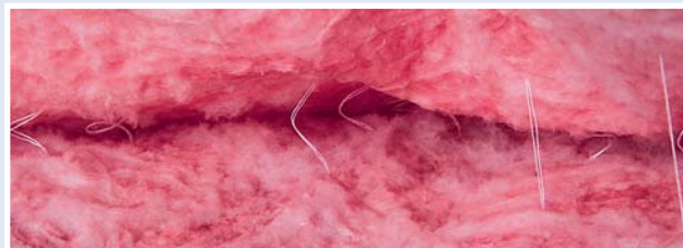
Fibre structure of microglass media
