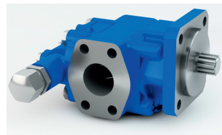
Optional Rickmeier product for Diesel engines: Fuel oil pump: R35/50 Appr. 70 dm 3 /min @ 1800 rpm Working pressure: 13 bar (max. 25 bar) Suction pressure: 0.6 bar abs. Kin. Viscosity: 4 mm 2 /s
