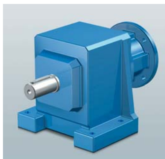
◀ MGS C Helical Gear Unit 10 sizes: C0 – C9 Rated torque: 21 – 7,000 Nm Gear ratio range: 2 – 300 Backlash: \leq 10 - 20 arcmin Particularly versatile with a variety of housing options
