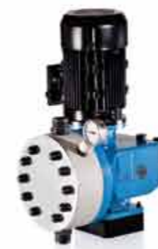
R410.2 ML Flow rate: 70 - 1200 l/h Counterpressure up to 16 bar
