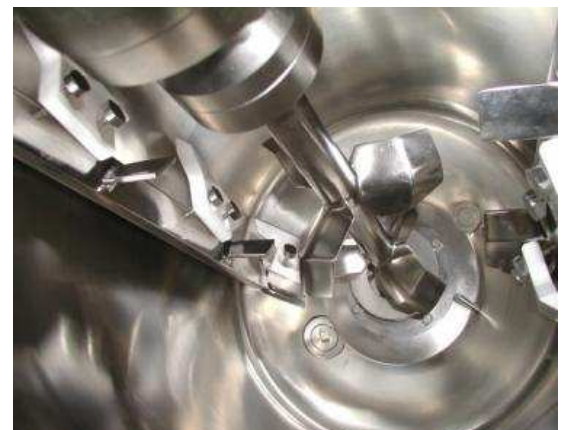
2 or 3 agitation independent movements for pastry products
