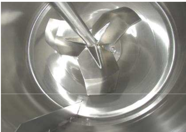
Three blades Agitator HTPG4™ for the mixing of fragile products
