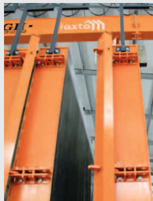
Modular side formwork
